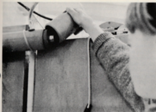
Top, the ultraviolet sterilizing setup, showing the cap of the ultraviolet tube and the inlet tube for water coming from the filters. (There are two of these.) At the opposite end are two outlet tubes plus an air vent with an overflow tube right on top. Bottom, general view of the setup for ultraviolet sterilization trial. The top tier is sterilized, the bottom is not.
