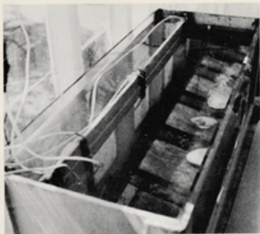
Another experimental tank. Filter medium is behind a partition, exposed to full sunlight through glass back of tank and unshaded greenhouse wall.
