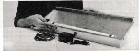
Completed conversion with fluorescent lamp in position.
