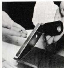
Remove plug from cord so that complete incandescent wiring can be removed from reflector.
