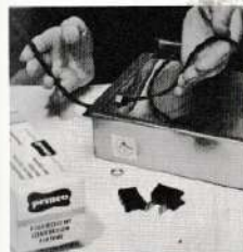
Remove plug from cord so that complete incandescent wiring can be removed from reflector.
