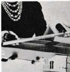
Knob and plug removed, and cord being unlaced from reflector.
