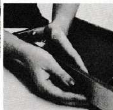
Remove knob and bolt which holds wiring.
